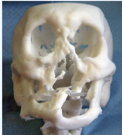
FIGURE 7-34. An anatomical biomodel was manufactured from CT scans using a fused deposition modelling (FDM) technique, a rapid prototyping or rapid manufacturing technology commonly used within CAD/CAM and engineering design.
